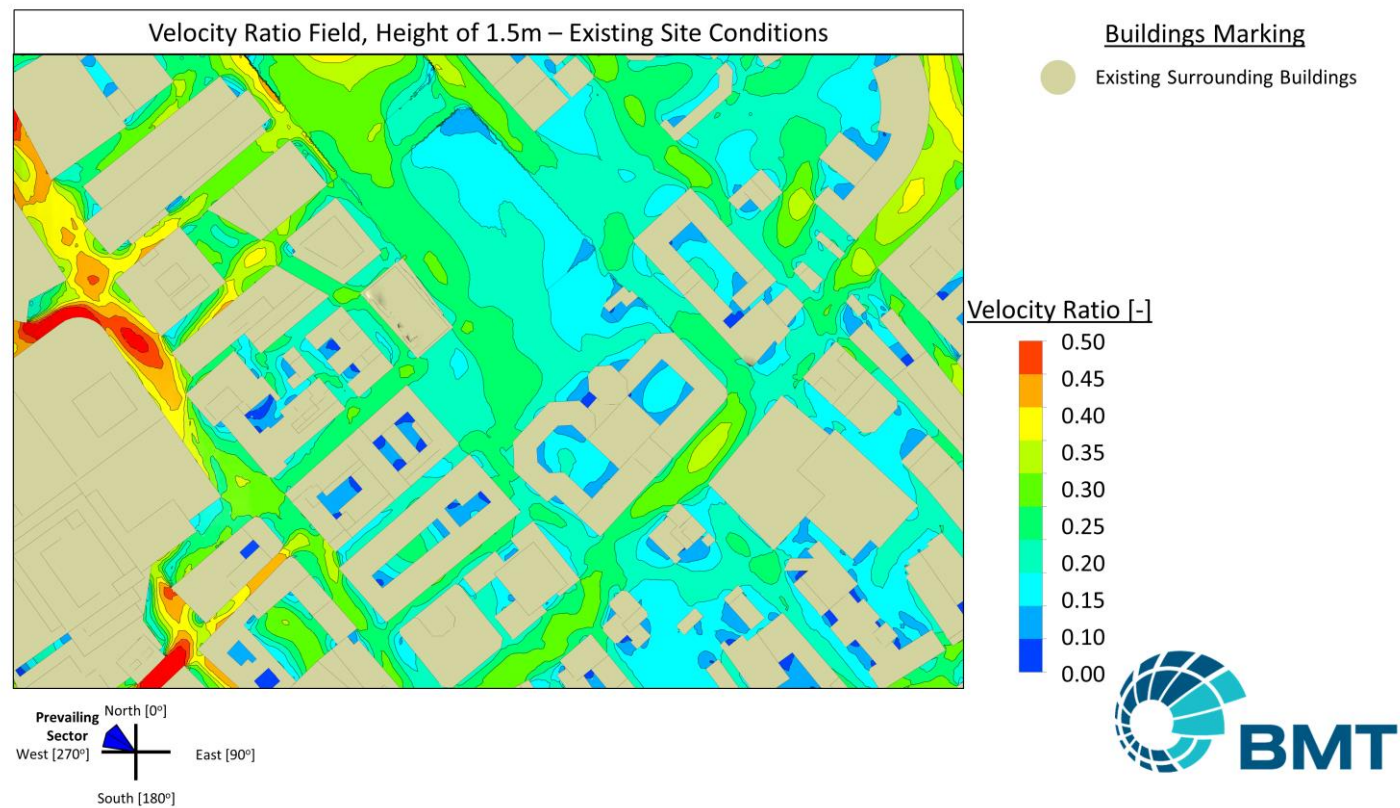
Figure D.1 - Velocity Ratio Contours at 1.5 m above Ground: Existing Site Conditions
