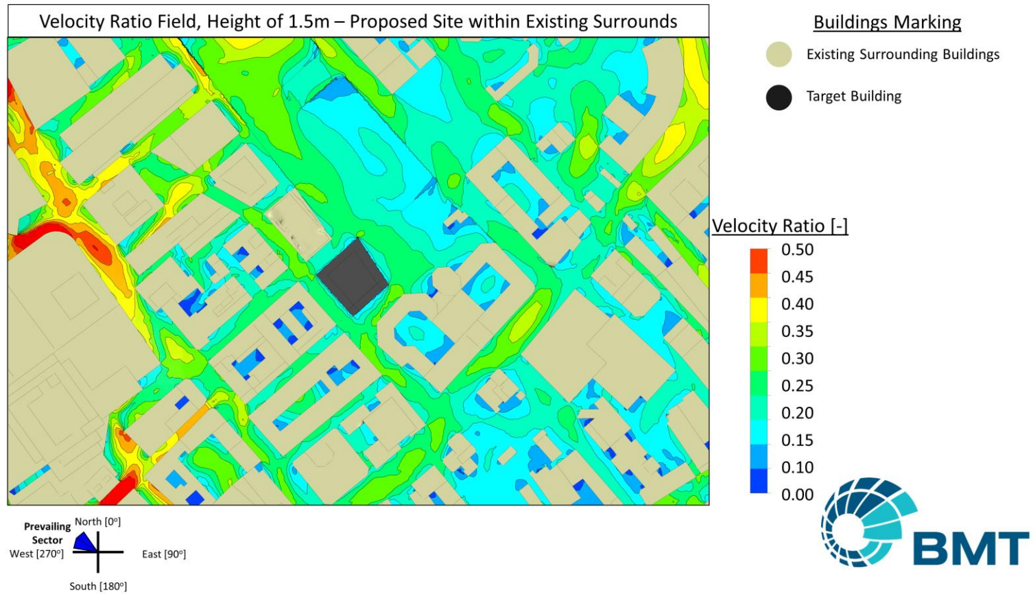
Figure D.2 - Velocity Ratio Contours at 1.5 m above Ground: Proposed Site, within Existing Surrounds
