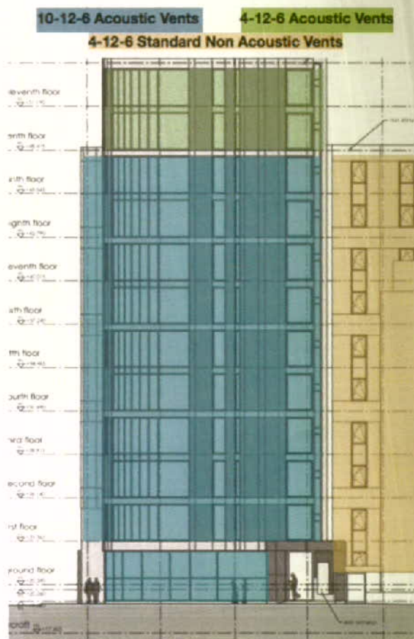
Figure 4: Proposed noise mitigation strategy - Hatton Gardens Elevation
