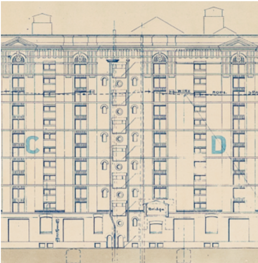
Original drawing of part of South elevation, showing larger openings at staircases and wire rope spans at 9th Floor level
