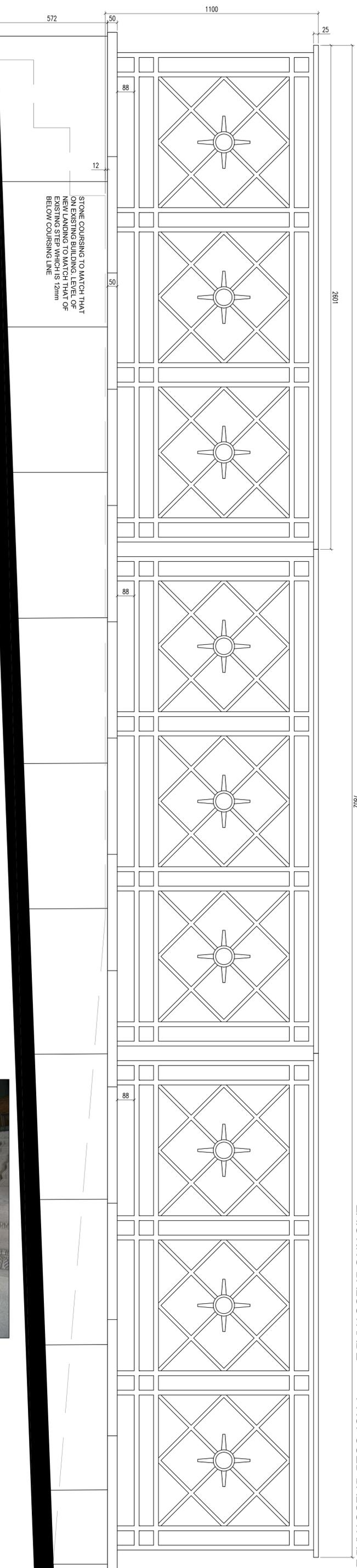
PROPOSED BALUSTRADE TO NEW RAMP, FORMED USING THREE SECTIONS FROM ROOFTOP BALUSTRADE
