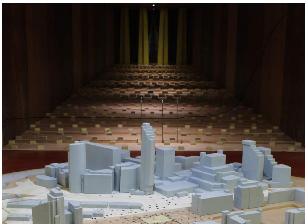
Figure 13.2: Roughness element and spires used in the wind tunnel to generate the upstream wind profile
