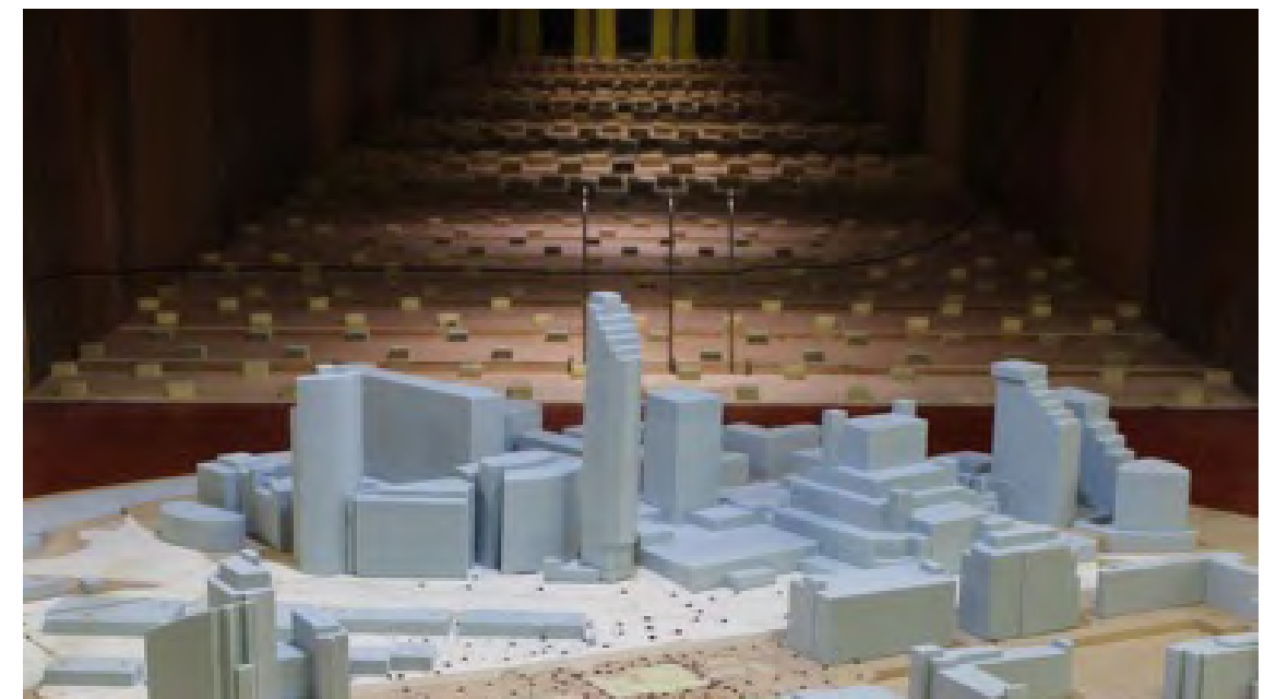
ROUGHNESS ELEMENT AND SPIRES USED IN THE WIND TUNNEL TO GENERATE THE UPSTREAM WIND PROFILE
