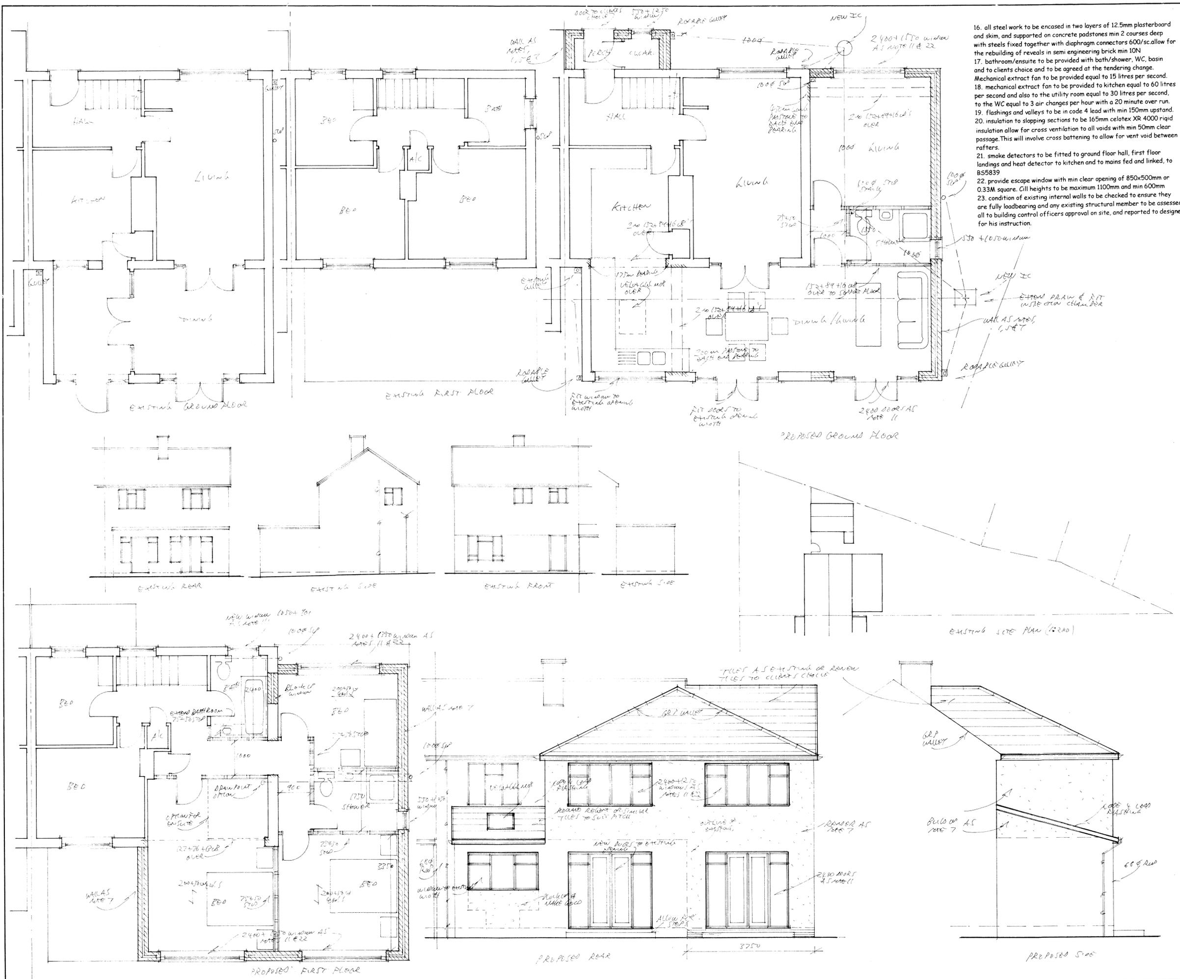
16. all steel work to be encased in two layers of 12.5mm plasterboard and skim, and supported on concrete padstones min 2 courses deep with steels fixed together with diaphragm connectors 600/sc.allow for the rebuilding of reveals in semi engineering brick min 10N
