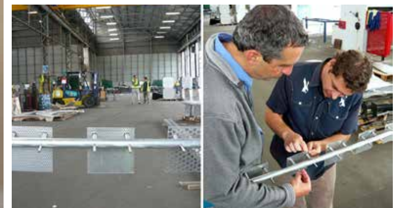
Photos of the full scale prototype show the curved profile and method of fixing which allows individual pixels to move independent of each other in a backwards/ forwards rotation.
