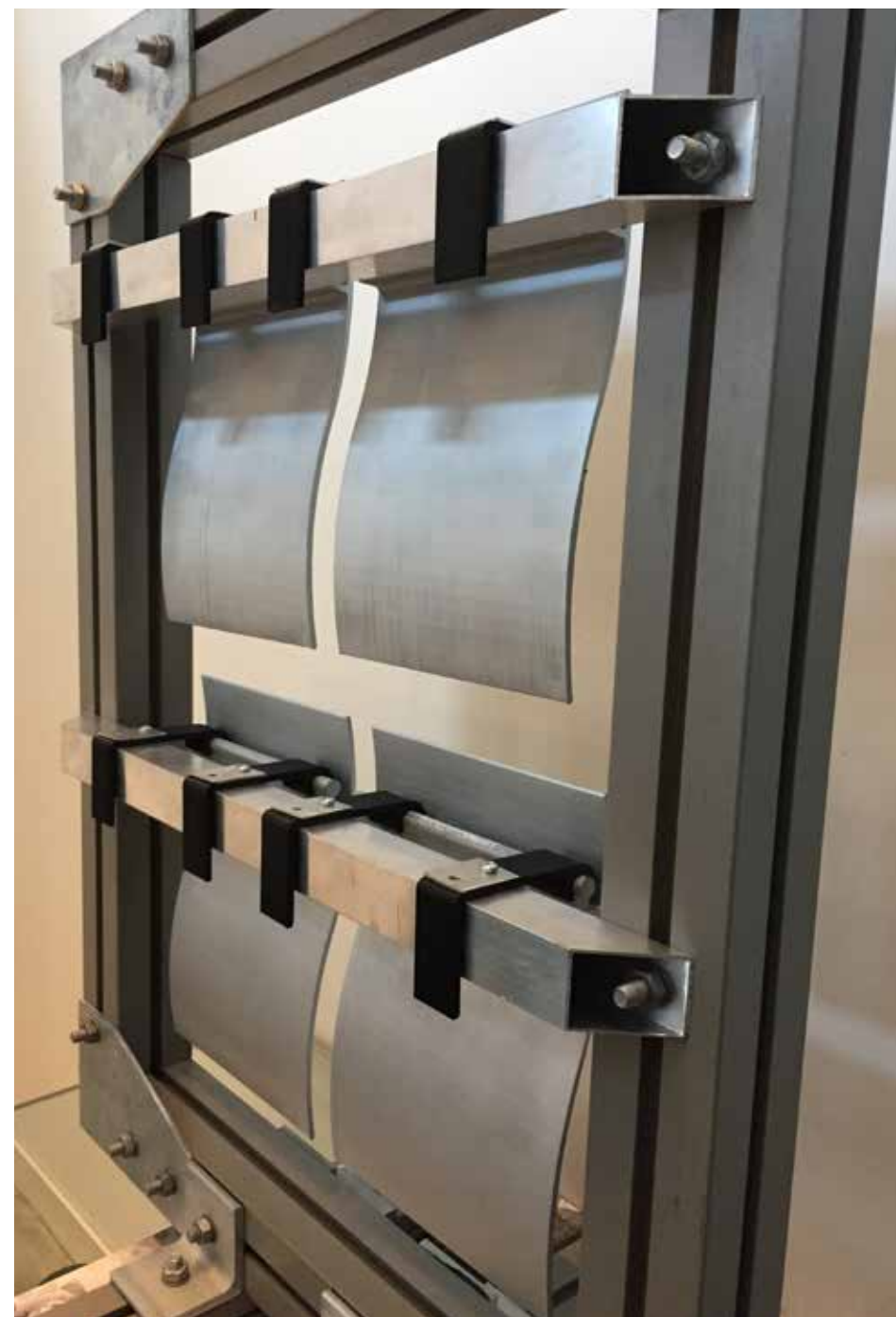
Photos of the full scale prototype show the curved profile and method of fixing which allows individual pixels to move independent of each other in a backwards/ forwards rotation.
