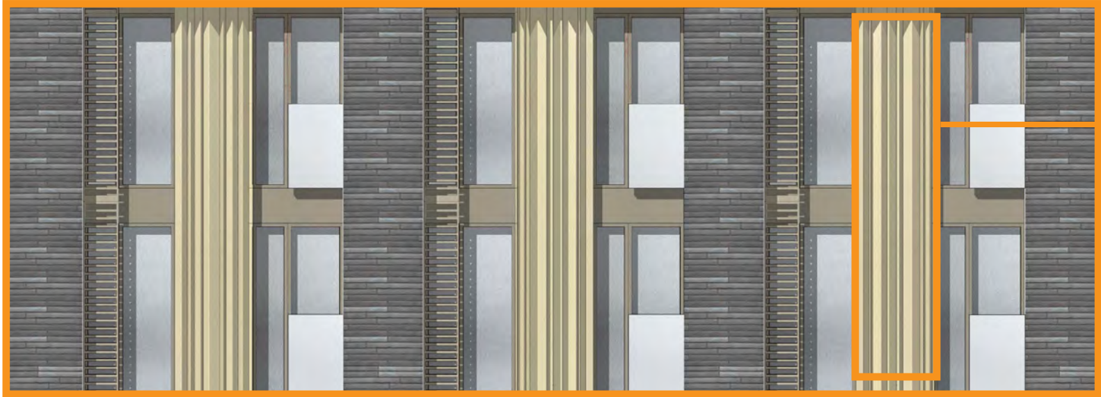
Aluminium panels are folded randomly to resemble hanged leather and add movement to the elevation.
