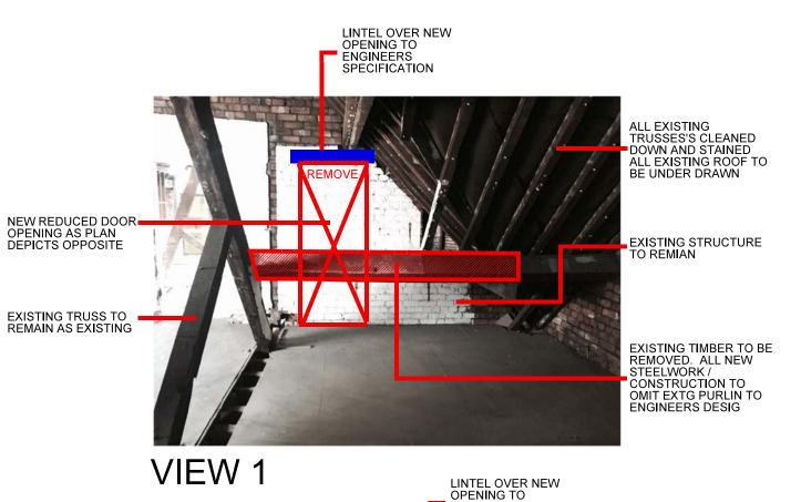
ENGINEERS SPECIFICATION ALL EXISTING TRUSSES'S CLEANED DOWN AND STAINED ALL EXISTING ROOF TO BE UNDER DRAWN
