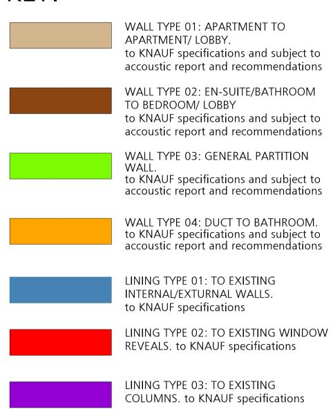
This drawing is to be read in conjuction with all relevant Architects, Engineers' and sub-contractor's drawings and specifications.
