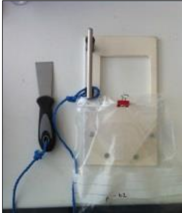
Figure 2-5 Wall sampling device for benthic invertebrates
