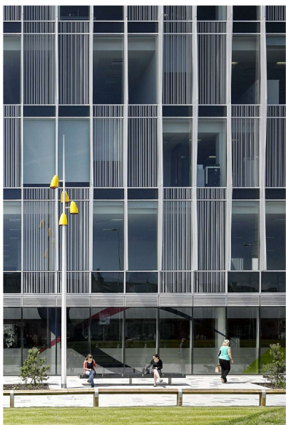
01 - Capless / Unitized Glazing System with fritted glass. System to intergal fins / solid, openable panels
