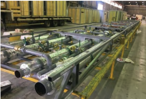
Mechanical and domestic riser modules for Block F, Imperial College London
