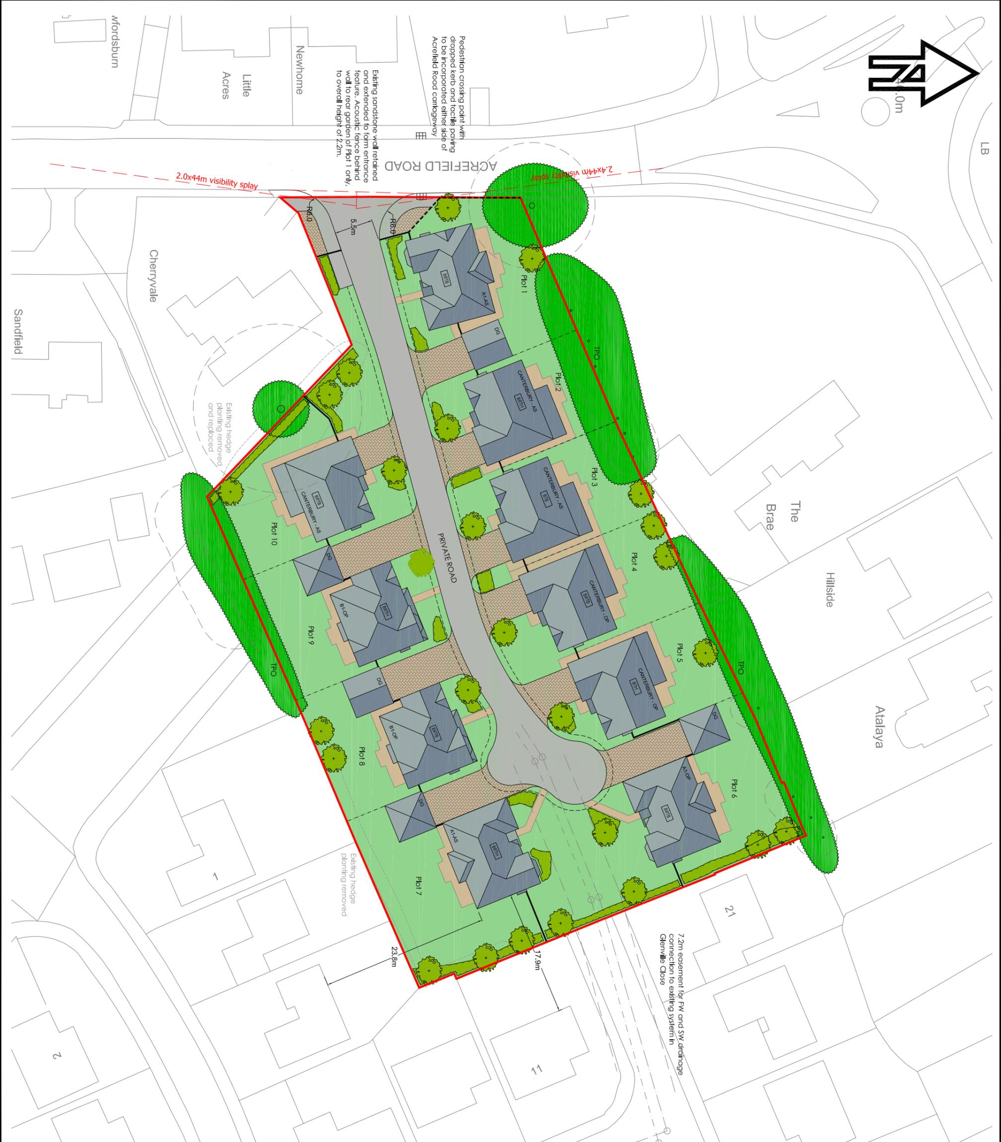
Existing sandstone wall retained and extended to form entrance feature. Acoustic fence behind wall to rear garden of Plot 1 only, to overall height of 2.2m.
