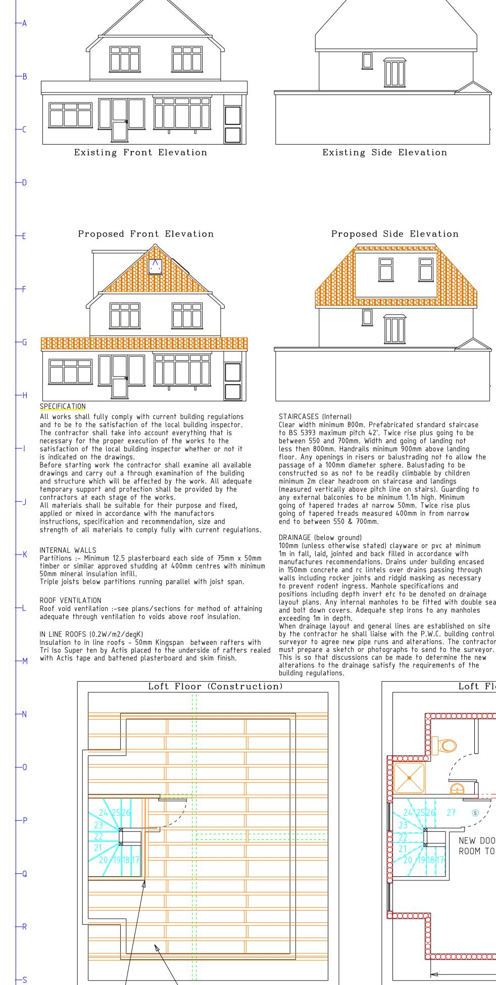
Floor joists 200 x 75 C24 grade
