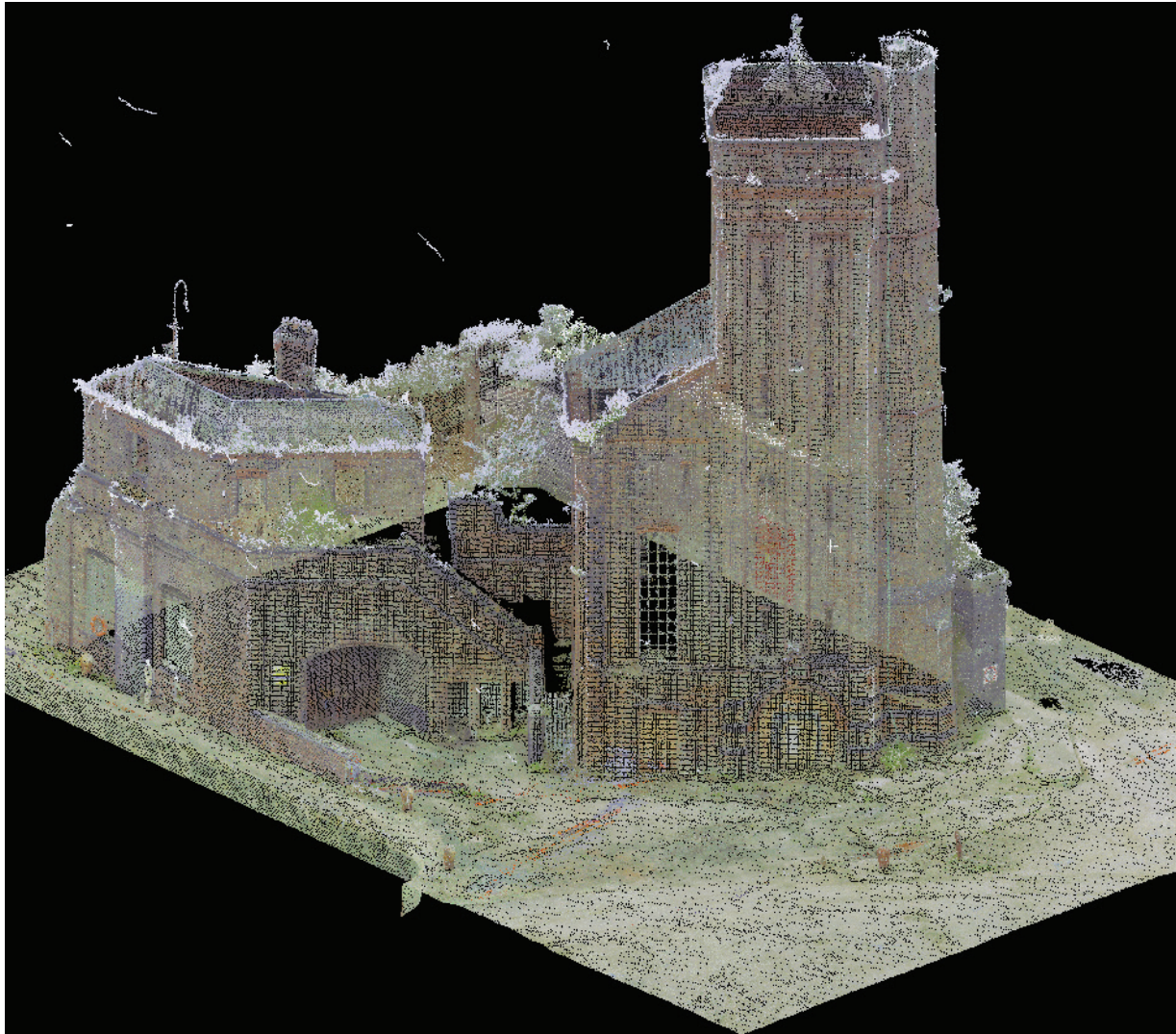
Partial Point Cloud Survey of Hydraulic Engine House
