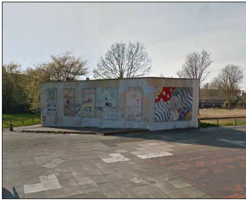
D – Ventilation shaft for adjacent railway tunnel.
