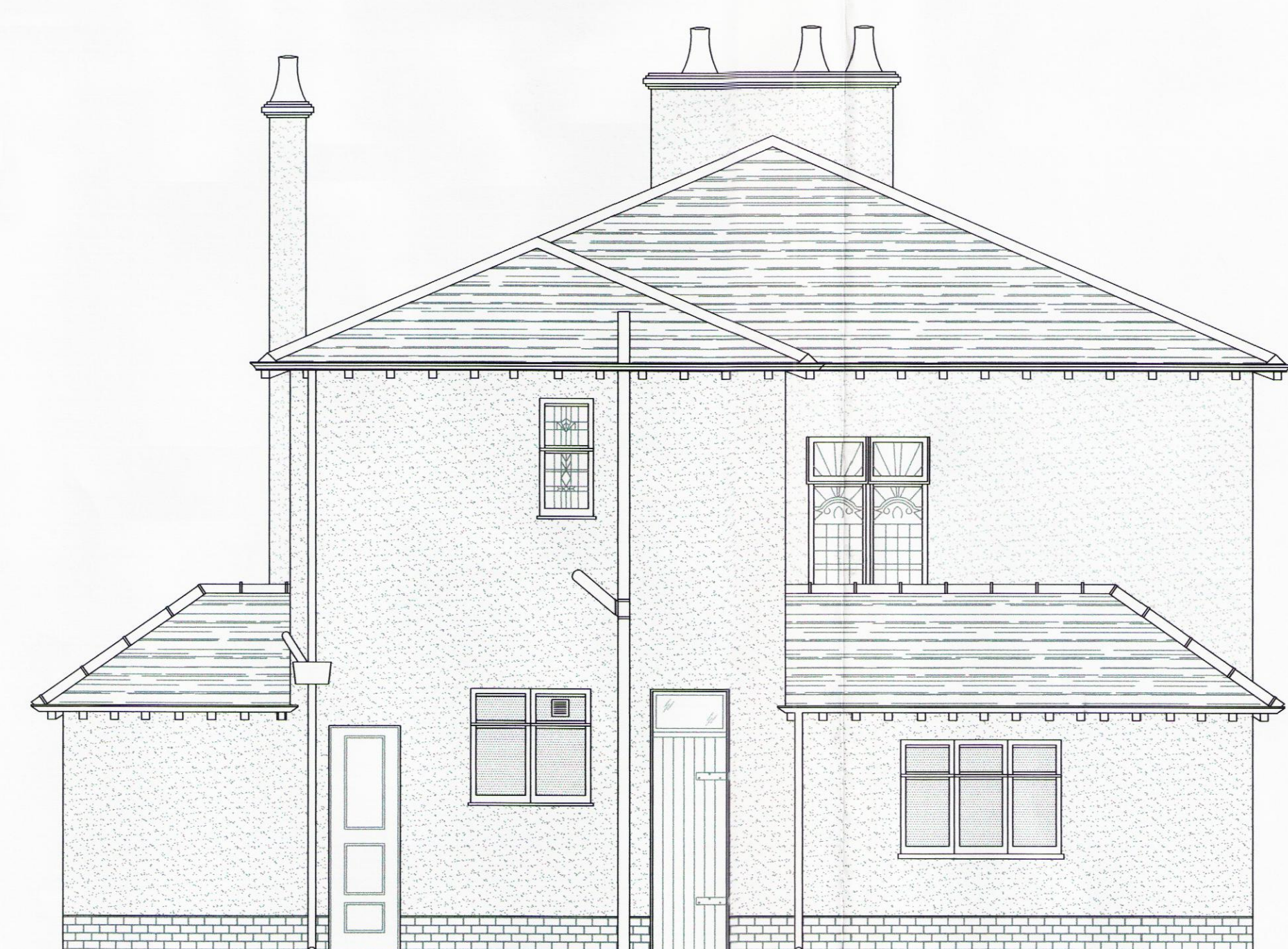
EXISTING SIDE ELEVATION SCALE 1:50
