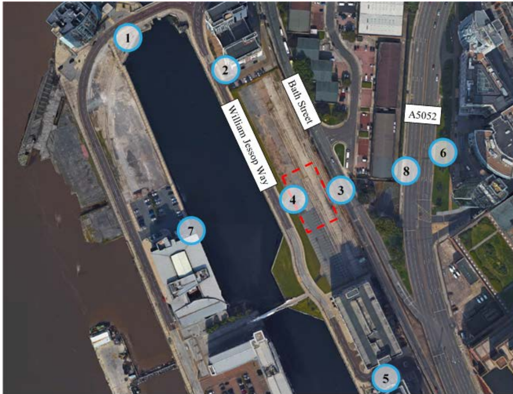
Figure C1: Site plan and noise measurement locations. Imagery ©2016 Google, map data ©2016 Google
