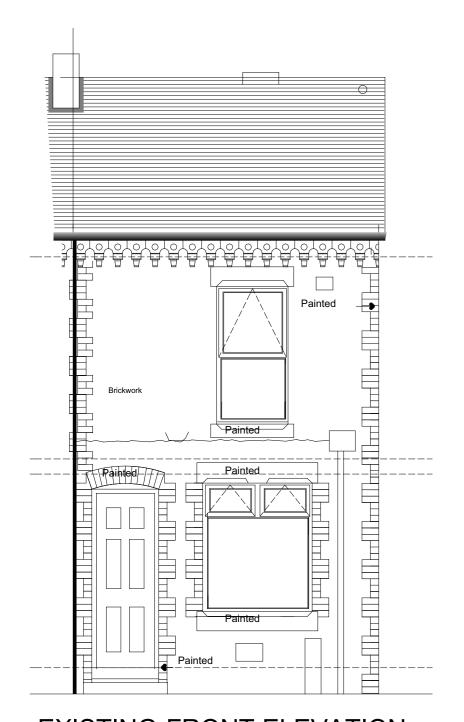
Brick Outrigg Outriggers to be demolished Note: Do not scale off this drawing. Do not rely on this drawing for purposes other than that stated 'Status'. Read this drawing with all project related Architects drawn and specified information including design risk assessments. Constructors must be familiar with the client's building asbestos register ahead of facilitating work contained on this drawing. Brickwork
