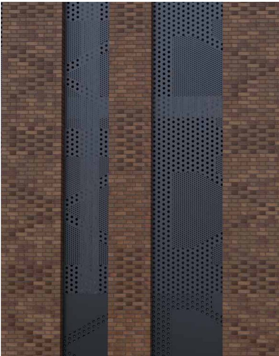
Figure 9.1.53: Visual illustrating selected bricks and the different perforations in the metal panels, creating an overall Leitch Truss pattern on the facade
