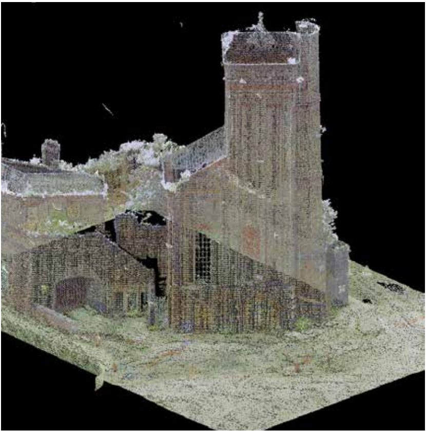
Figure 6.8.2: Point cloud of Hydraulic Engine House produced from ground survey
