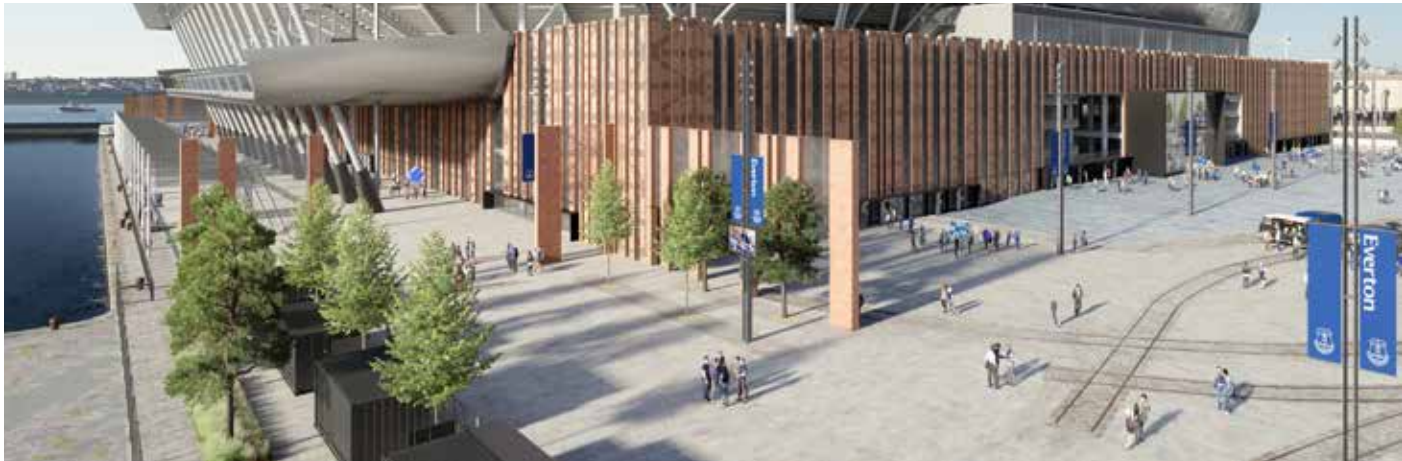
Figure 7.3.6: Proposed wind mitigation elements at south-east corner of stadium
