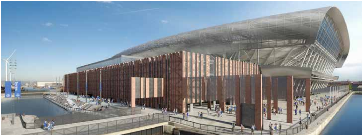
Figure 7.3.5: Proposed wind mitigation elements at south-west corner of stadium
