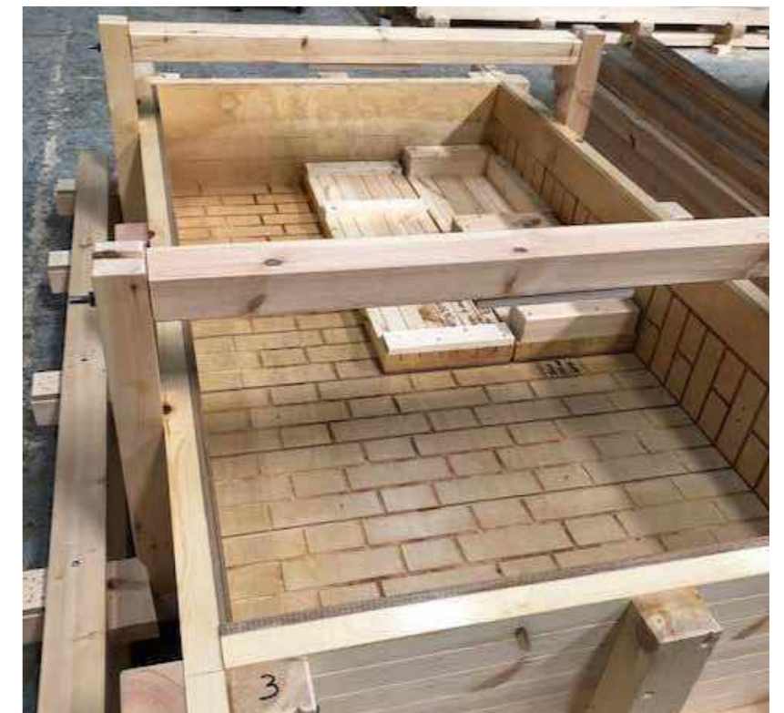
Images of the formwork for the concrete panels which will receive the bricks
