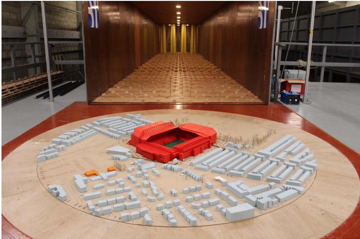
Figure 12.34 Proposed Scheme with Existing Surrounding Buildings and Existing Landscaping Scheme (Configuration 2) – View in the Wind Tunnel (from the south)
