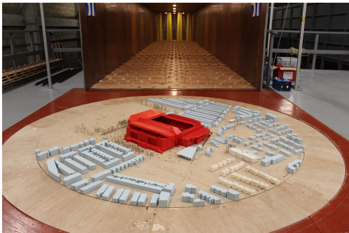
Figure 12.37 Proposed Scheme with Cumulative Surrounding Buildings and Existing Landscaping Scheme (Configuration 3) – View in the Wind Tunnel (from the west)
