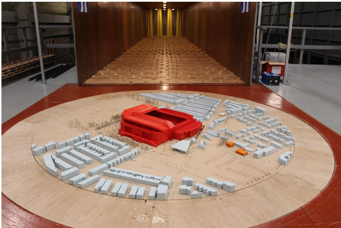
Figure 12.35 Proposed Scheme with Existing Surrounding Buildings and Existing Landscaping Scheme (Configuration 2) – View in the Wind Tunnel (from the west)
