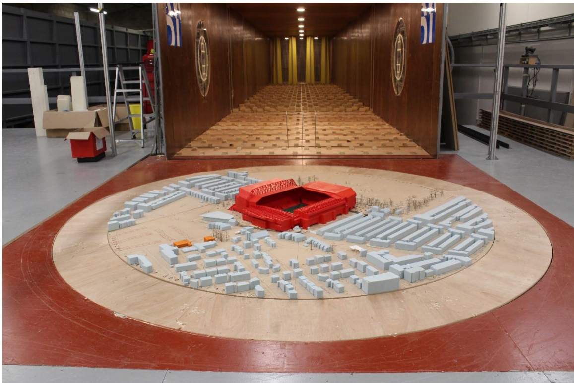
Figure 12.38 Proposed Scheme with Existing Surrounding Buildings, Existing and Proposed Landscaping Scheme (Configuration 4) – View in the Wind Tunnel (from the south)
