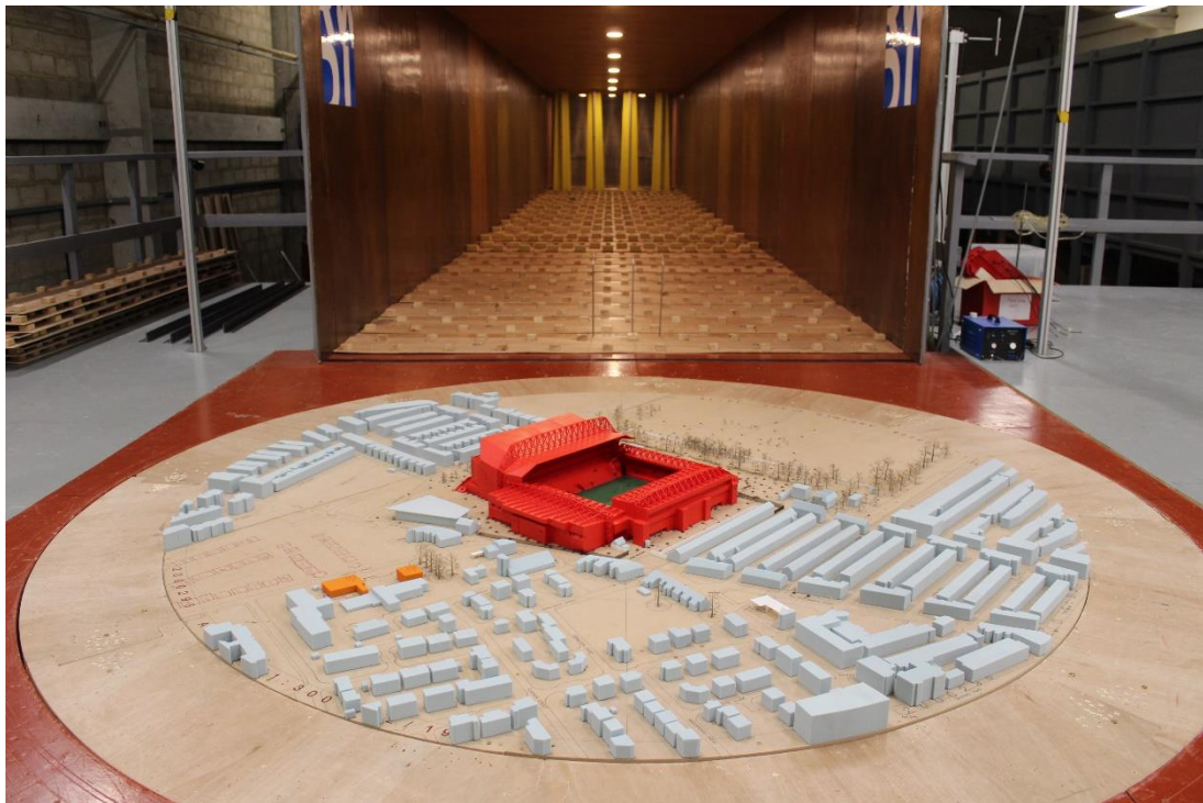
Figure 12.32 Existing Site with Existing Surrounding Buildings and Existing Landscaping Scheme (Configuration 1) – View in the Wind Tunnel (from the south)
