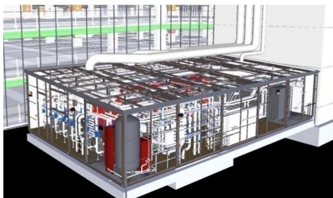
Example of an offsite-modelled plantroom.
