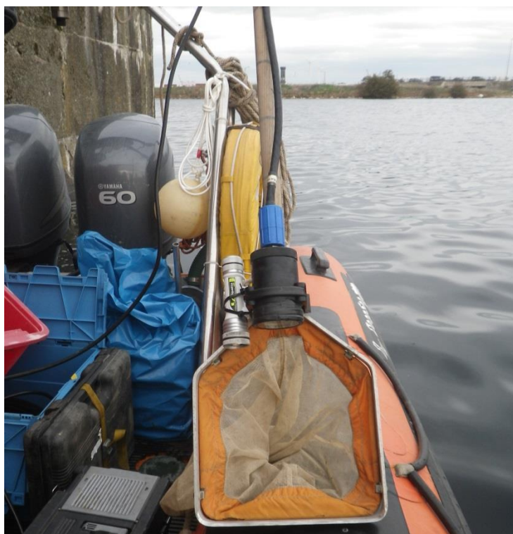
Fig. 3. Photograph of the net used to scrape the sides of the dockwall showing the attached underwater video camera.
