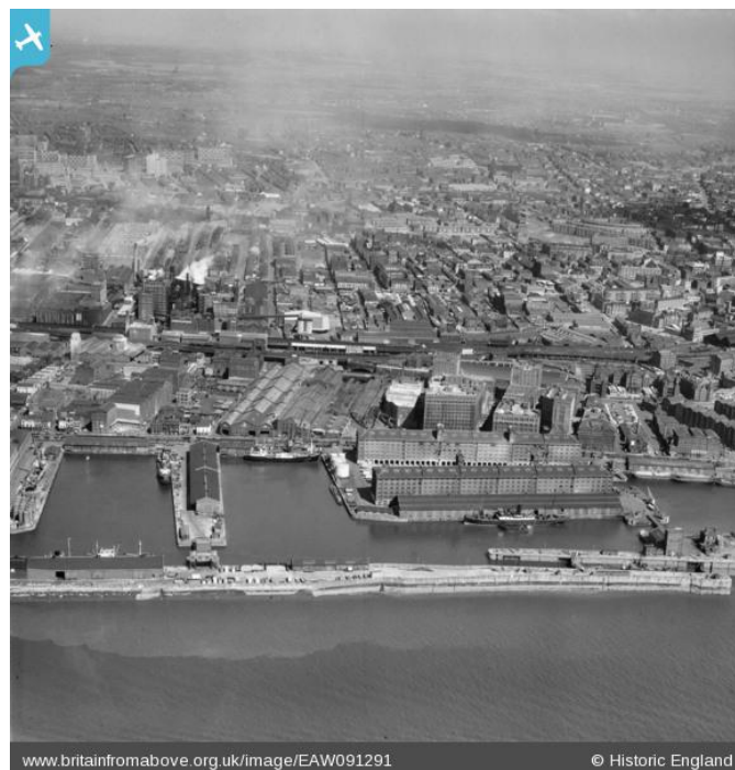
Figure 9.10: 1949-West Waterloo Dock has been re-configured with the addition of the river lock, and the re-building and change in orientation of the sea wall. The northern quay wall to West Waterloo Dock has been removed. (Historic England).
