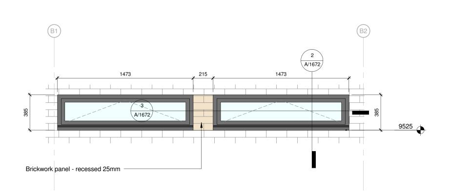
01 - Toilet Windows With Recess Brickwork Panel - Details
