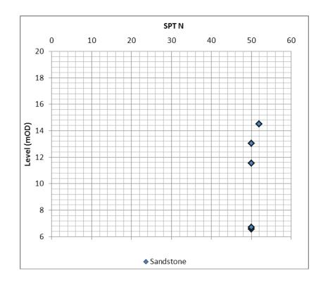
BS8002 suggests a friction angle,  $\Phi$ ' of 42°. For design purposes a characteristic value  $\Phi$ ' of 40° will be adopted. Effective cohesion, c' will be taken as 0kPa.
