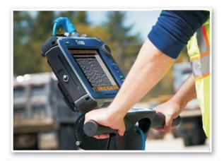
The SIR® 4000 is GSSI's first high-performance GPR data acquisition system designed to operate with analog and digital antennas. This evolutionary step allows true versatility and flexibility by supporting a wide range of users, beginner to advanced, in numerous applications.
