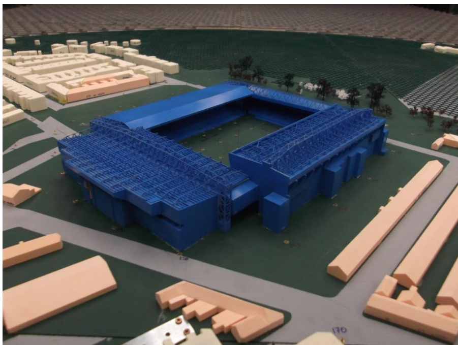
Figure B.3 - Wind Tunnel Models of the Proposed Development, Viewed from South, Wind Tunnel Set-Up, Close Up View, Existing Configuration
