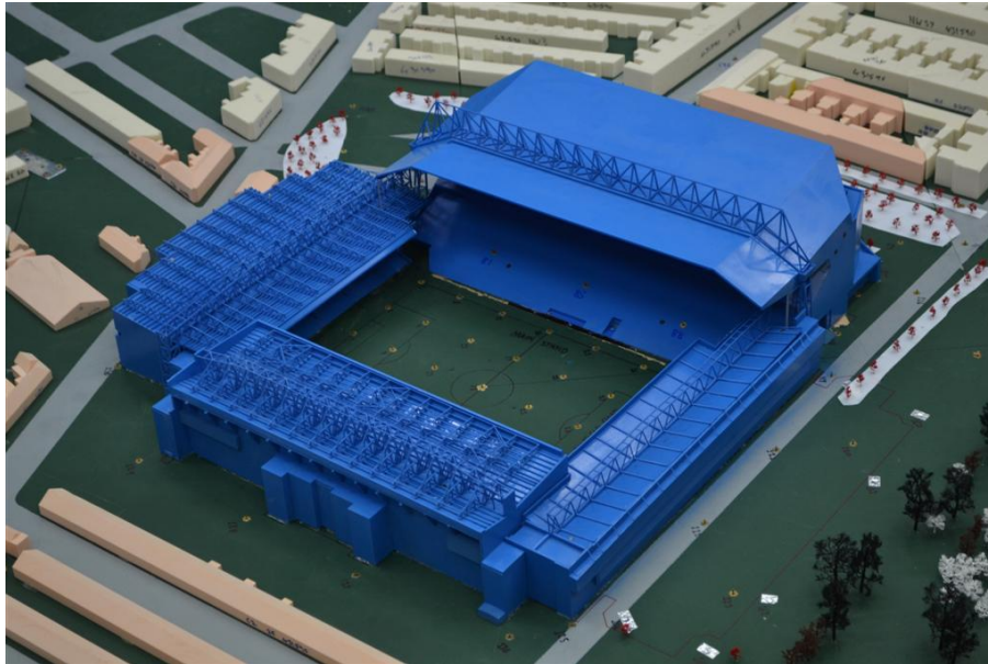
Figure B.7 - Wind Tunnel Models of the Proposed Development, Viewed from North, Wind Tunnel Set-Up, Phase 2
