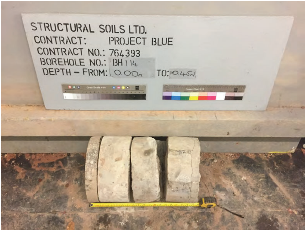
BH114 - Concrete Core
