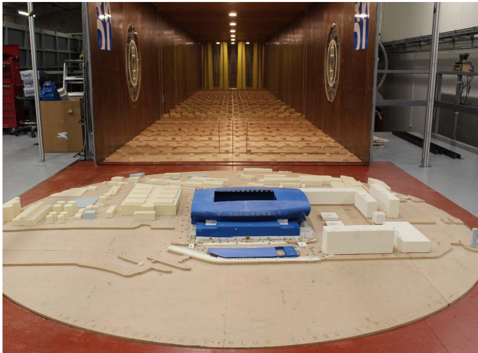
Figure 45: Proposed Development with Cumulative Surrounding Buildings, Proposed Landscaping Scheme, Design Interventions and Mitigation Measures (Configuration 4) – View in the Wind Tunnel (from the West)
