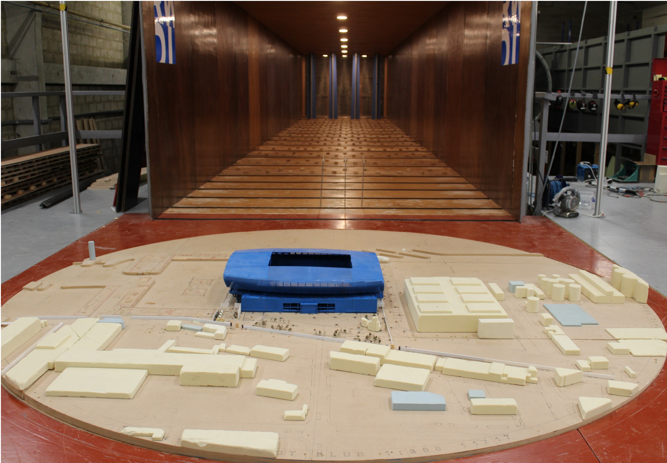
Figure14.1 Proposed Development Model in the Wind Tunnel
