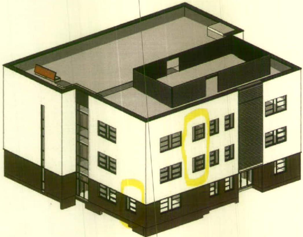
4. Whilst not fully resolved, we are looking to mechanically ventilate the refurbished music department adjacent to the new main entrance. Because of existing building height restrictions, we will have to run the ductwork on the roof. As a result, we may also need a
