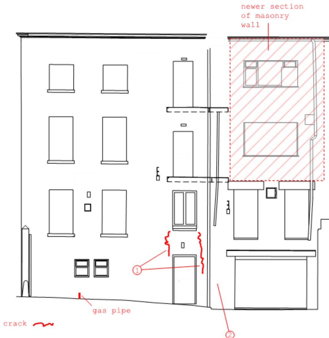
Figure 3 – EP building West Façade Elevation Defects
