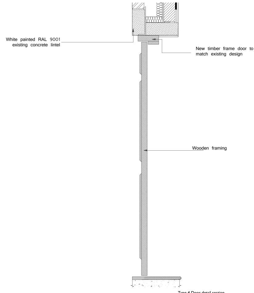
Type 4 Door detail section scale 1.10
