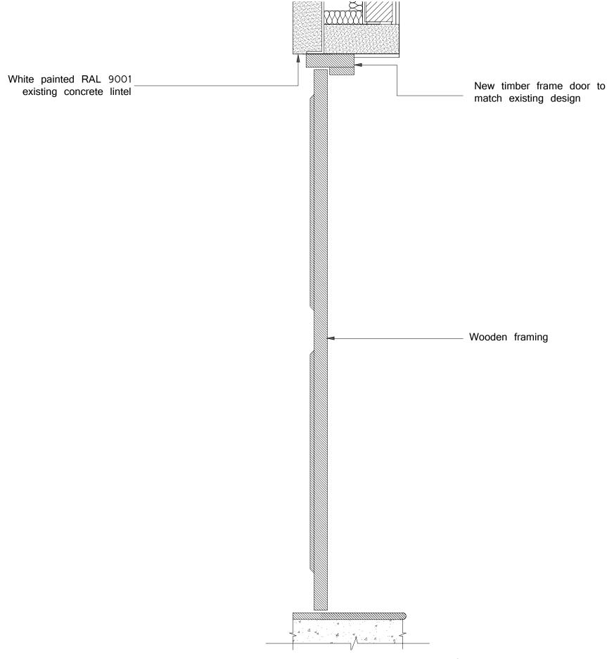
Type 2 Door detail section scale 1.10
