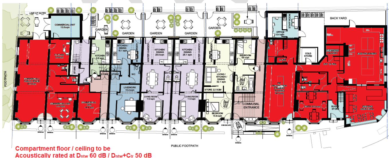
Figure 3: areas of floor / ceiling where enhanced sound insulation is recommended
