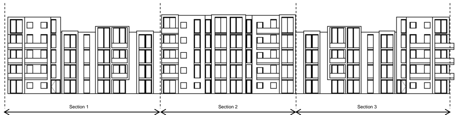
Block 1 is divided up into 3 separate sections within the whole block, each having their own circulation cores
