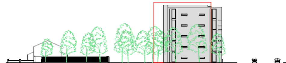
Position and scale of the old scheme is outlined in red against the revised scheme which is smaller and further back/closer to Upper Parliament street than the original design was
