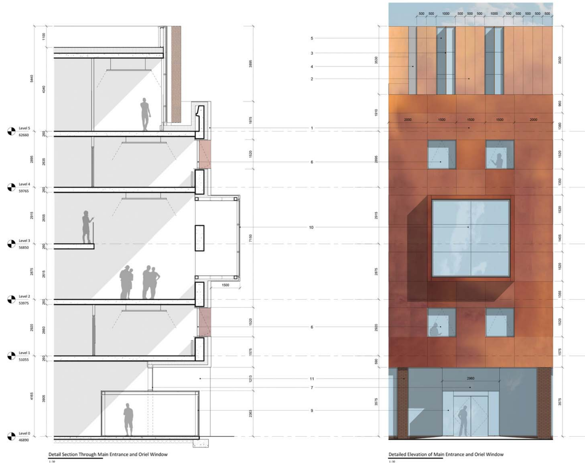
Detailed elevation and section through the new entrance lobby and oriel window
