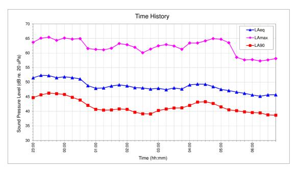
The lowest 15 minute background noise level is 39 dB L<sub>A90</sub>. We will use this as our design target (although BS4142 does not require the lowest level to be used, we do so here as a worst case).
