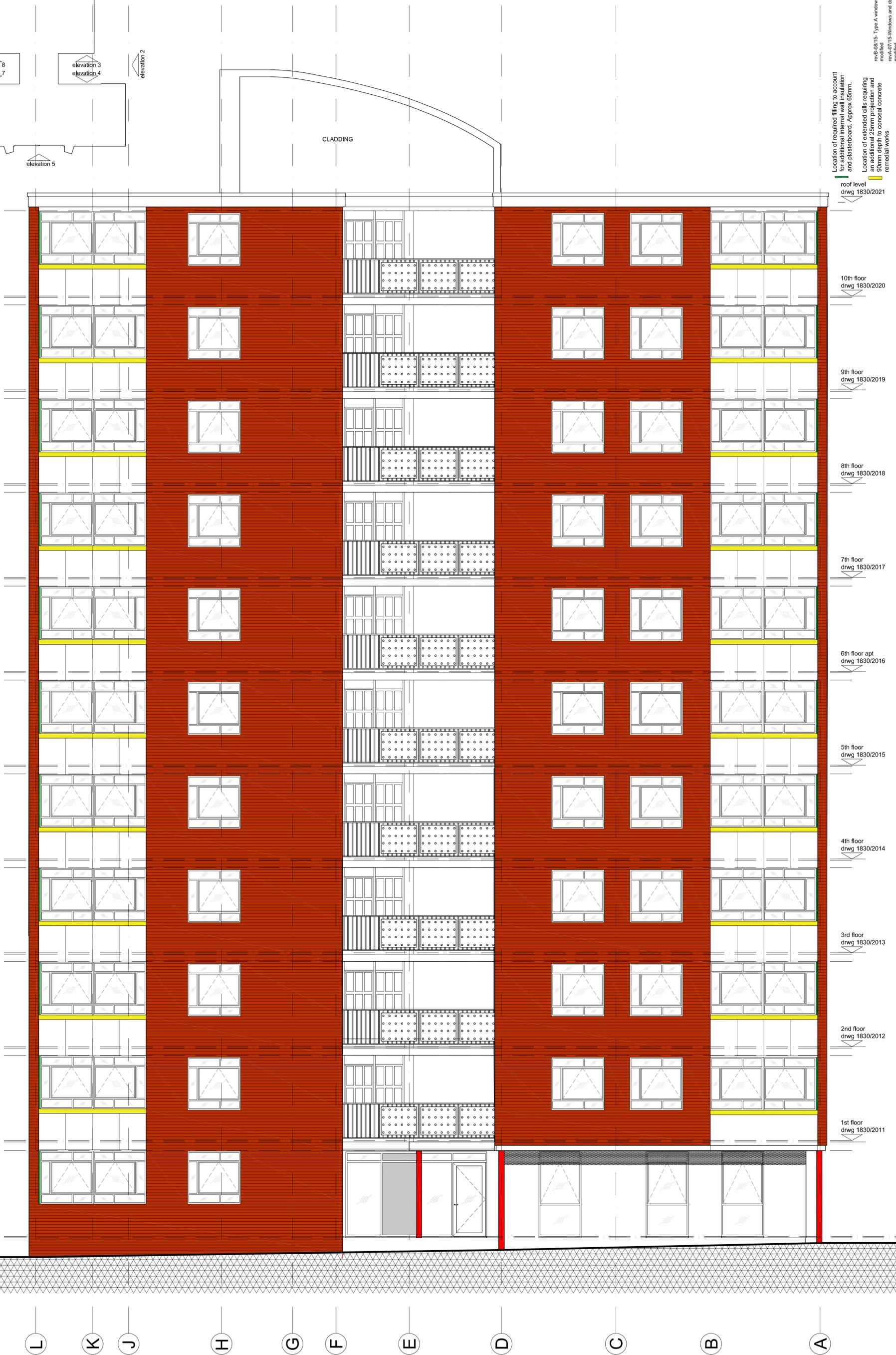
Location of required filling to account for additional internal wall insulation and plasterboard. Approx 65mm.
