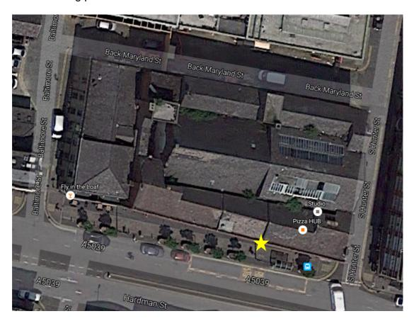
The microphone was on a boom outside a first floor window and clearly represents the general noise on Hardman Street. Brief measurements were also made on S Hunter St and Baltimore St, simply to verify calculated levels in these side streets.
