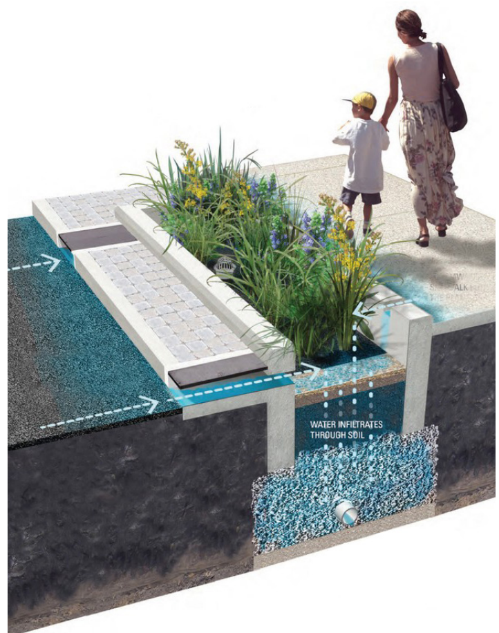
Diagram of a typical rain garden system
