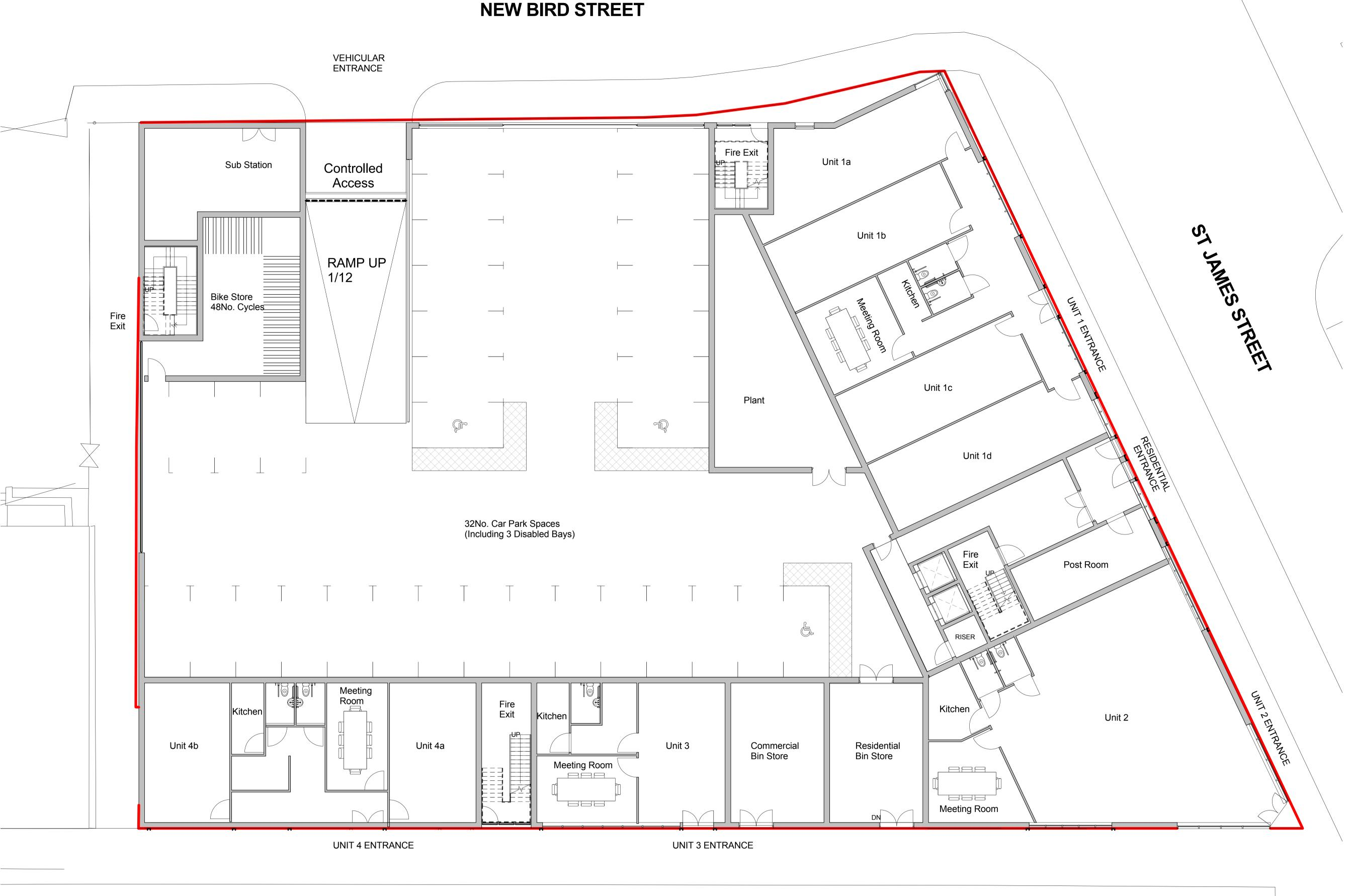
Lower Ground and Ground Floor Plan
