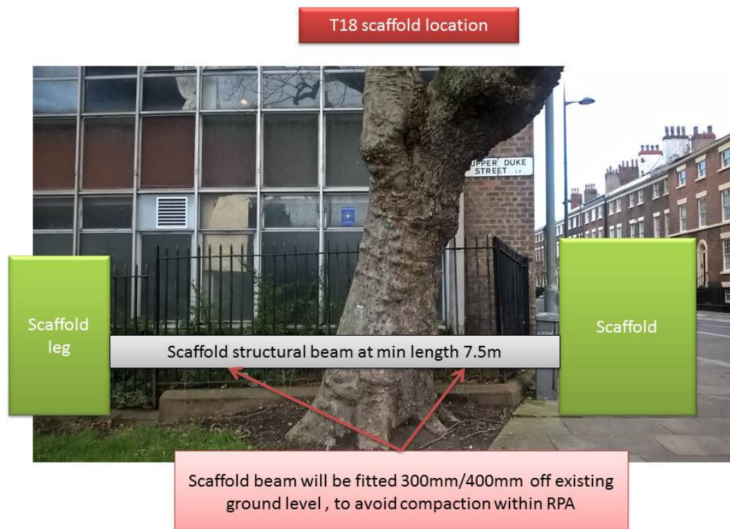
Figure 8 : Temporary Ground Protection Measures to allow scaffold erection within CEZ to Tree T18
