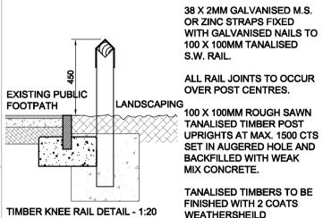
TANALISED TIMBER POST UPRIGHTS AT MAX. 1500 CTS SET IN AUGERED HOLE AND **BACKFILLED WITH WEAK** MIX CONCRETE.
