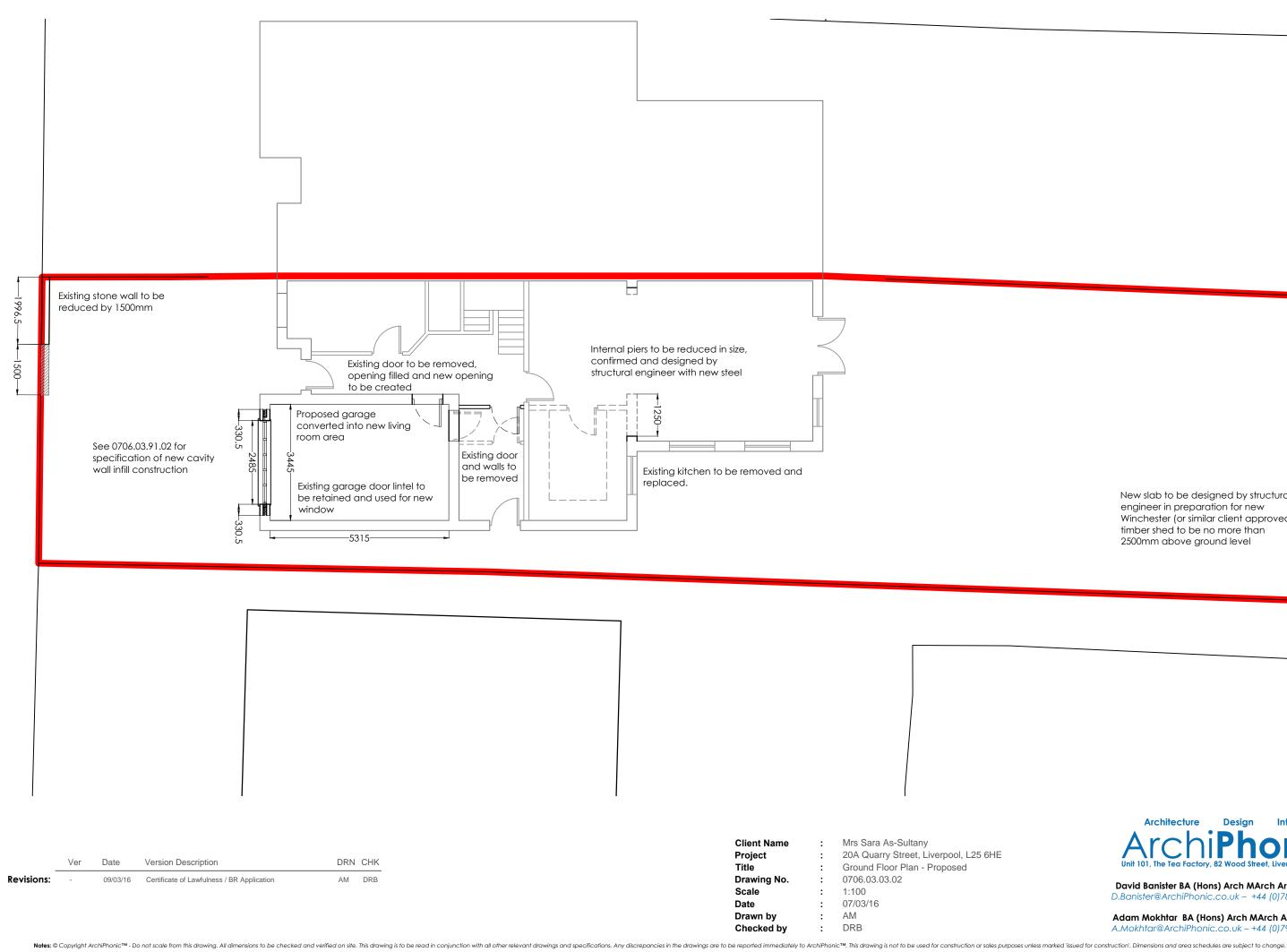
New slab to be designed by structural engineer in preparation for new Winchester (or similar client approved) timber shed to be no more than 2500mm above ground level
